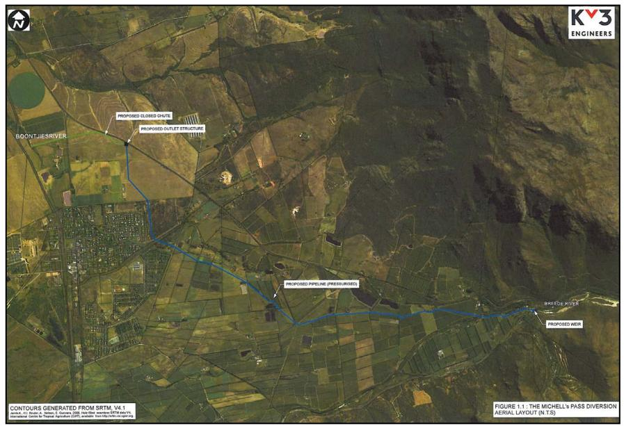
Figure 4.3 The proposed general layout of the Michell's Pass diversion scheme
